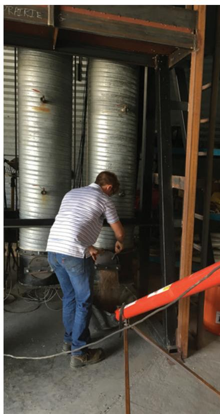
*Unloading lentils from the 15 bu test bins at the end of the drying trial.*
