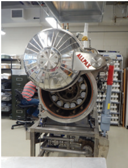
Cans in retort for processing at Bean Pilot Plant at the AAFC Lethbridge Research and Development Centre. Photo courtesy of Parthiba Balasubramanian.
